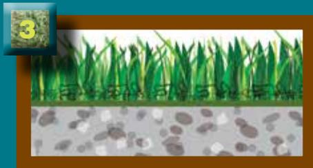
Lay your Newturf lawn grass, making sure you start from one edge and roll out. Cut the overhanging quantities with a sharp knife. Remove the 'salvage', black strip, from both sides of the grass. This cannot be used to join the grass.
