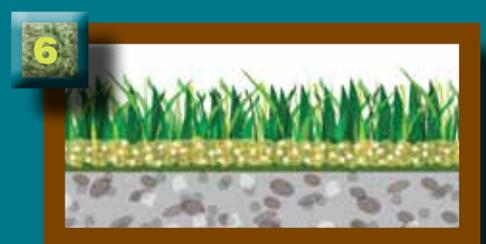
Top dress the grass with an even sprinkling of fine, dry "eco-fill" silica sand to a thickness of 15-20mm. A broom can be used at this stage to sweep in the sand evenly and to also brush the grass blades straight and vertical.
