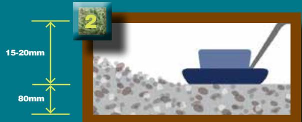
Lay 80mm of crushed roadbase and compact with vibrating plate. The level of crushed roadbase, when compacted, should be 15-20mm below "finished height" of surrounding edging/paving
