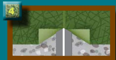
To join rolls/pieces of grass, use the Qualtape. Place the silver side of the qualtape onto base, this will leave the split white side facing up. Remove one side of the white cover and stick the grass to this, then repeat the process for the other side.
