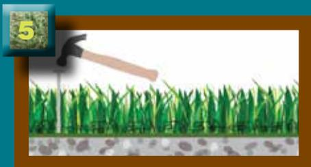
Once you have covered the complete area, simply nail all of the perimeters down at 500mm intervals using 150mm flat head nails. This must also be applied to the joining seams.
