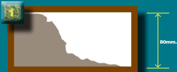
Using a rope or hose, layout the proposed area. Excavate the area to a depth of 80mm. Sprinklers may be capped or removed at this stage.
